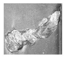
Holes in boiler wall caused by corrosion
