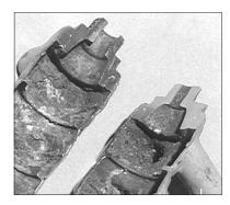
Radiator clogged with sludge (sectioned)
