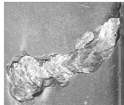
Holes in boiler wall caused by corrosion
