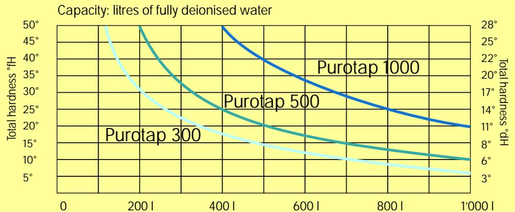
**Usage** When using Purotap, the installation is only filled with that amount of fully deionised water to guarantee compliance with the limits stipulated in today's directives for total hardness, conductivity and neutral salts.
