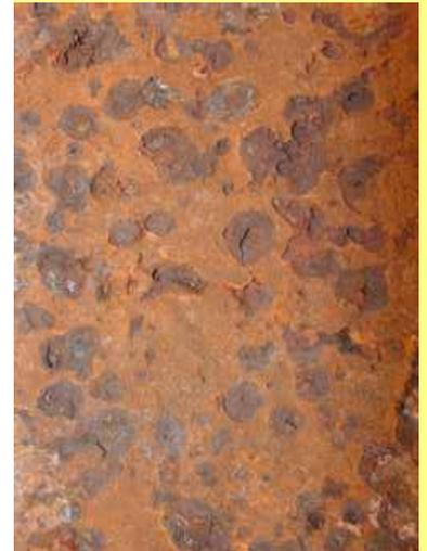
Localised corrosion for high levels of salt
