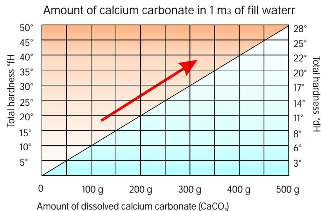
According to Swiss directive SWKI 97-1 and other European standards, the water used to fill systems of capacity up to 1 m<sup>3</sup> must be softened if its hardness is 35° f or more, reducing to 30° f for systems of capacity greater than 1 m<sup>3</sup>.
