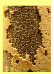
Limescale in the heat exchanger
