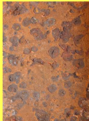
Localised corrosion for high levels of salt
